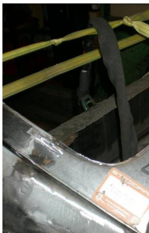
leak and also due to water coming in through the gas filler lid. You start to see the weak points when you completely disassemble a car. If the boot that goes around the gas filler tube to the tank leaks it goes right into the inner structure under the luggage area liner (carpet).
