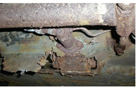
the interior. After more investigation, I discovered the driver's rear quarter panel had been replaced sometime in the past due to a rear collision, and quarter windows were leaking due to a less than stellar repair. The water ran down and actually rusted both the outer and the inner panels. The repairs had to be done in sections both in and out to maintain the structural integrity.
